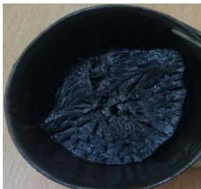
Figure 1. Manganese ferrite ( \text{MnFe}_2\text{O}_4 ) obtained by sol-gel autocombustion method
